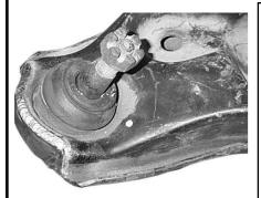
NOTE: The lower factory control arms must be trimmed and boxed for clearance to the brake rotor. Check clearance thru the entire suspension movement and lock to lock steering range. When vehicle is on jack stands it will appear to have clearance but will interfere when the suspension is bottomed out.
