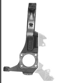
The spindle modifications required for the 75200/75250 brake kits are shown above. The faintly displayed material should be removed. Spindles can also be sent to Mark Williams Enterprises to have these modifications performed. If you have any questions call 303-665-6901, fax 303-665-7021 or e-mail to info@mark-williams.com
